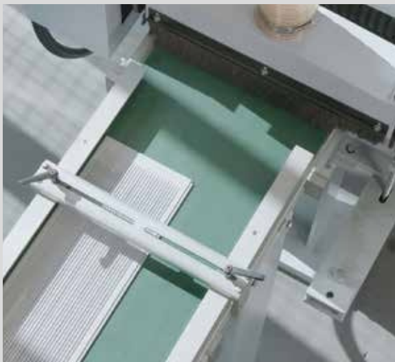
By using a grooving unit, grooves are milled on the backside of the floorboard
